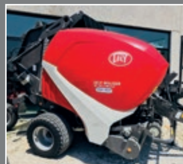
Rotopressa Lely 160 V master 13 coltelli centralina e link pick-up largo camera variabile
